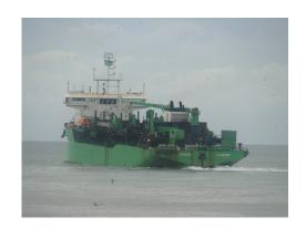
At low tide, it scoops sand from the bottom of the sea and stores it in the hold of the ship.
