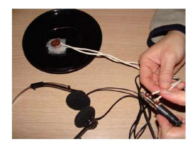
Finish off by placing the other coin with electric wire taped to it on top of the stacked materials. Attention! The copper filaments on the last coin should be facing up!.
